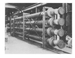
Crystallization is a "one way" process. There are no repeated evaporations and condensations to effect purification. Latent heats of fusion are very low, making total utility costs low. Cooling crystallizations may be done without costly vacuum system, or other complex and energy intensive auxilliary equipment.
